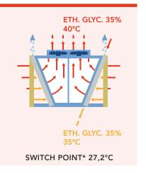
(\*) Fans at 1.100 RPM (Jumbo for fans 910 mm)
