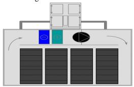
**Max airflow** 4x4m/2 16,000l/s ESP 200Pa est **Dehumidification capacity**
