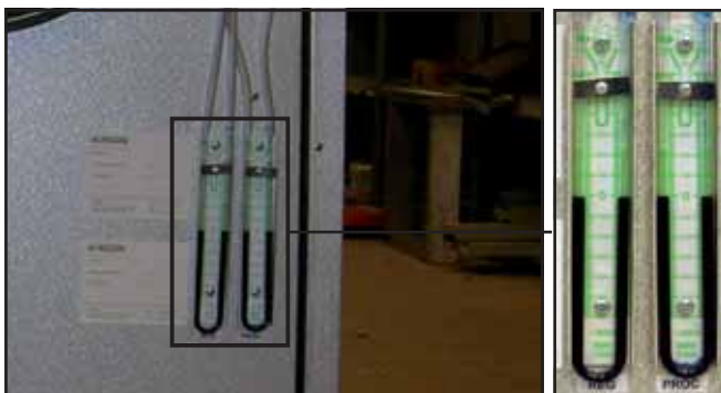
FIGURE 7: E.g. Differential U-tube manometers setup
